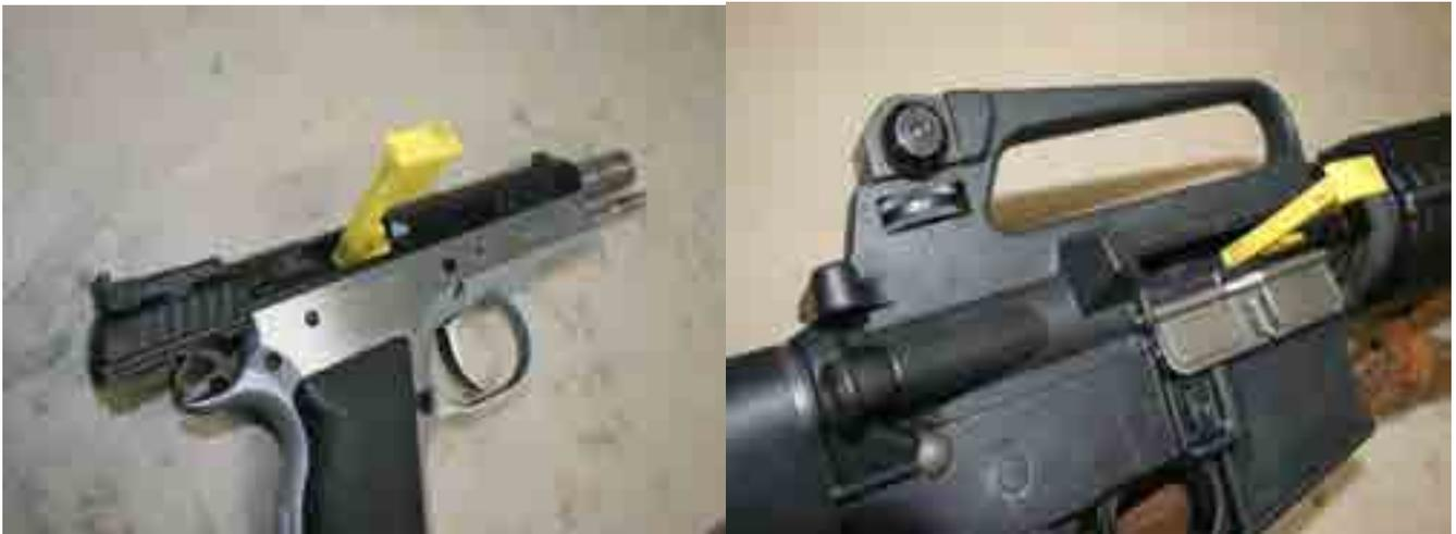
**Figure 12. Examples of properly installed Empty Chamber Indicators**
